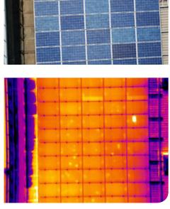
Example of PV module defects detected by FLIR Ax5 camera
